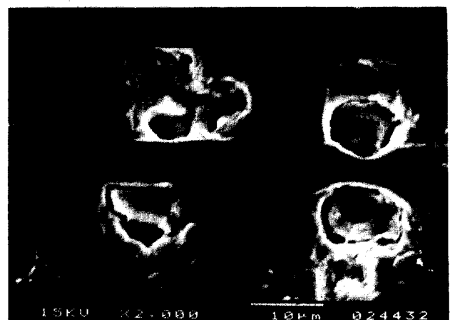
Fig. 2. Electron micrograph showing fibre/matrix interaction in a freeze-gelled Nextel/silica-zirconia ceramic-matrix composite during sintering at 500°C following infiltration.
