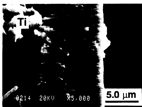
Fig. 1. A representative micrograph of the reaction layer obtained by treating \text{B}_4\text{C} in Ti powder ( 1100^\circ\text{C} , 6 h), cross section.
