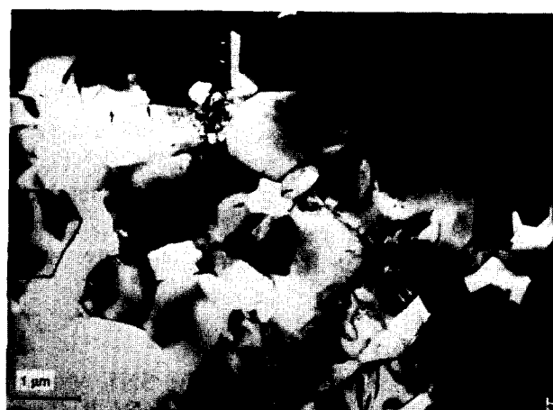
Fig. 5. Corroded SN2: typical planar view regions at the corrosion zone interface after corrosion for 800 h; arrows indicate intergranular voids foreign to the uncorroded microstructure.
