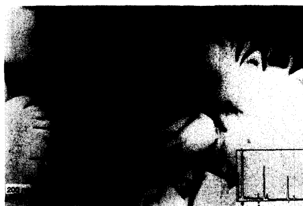
Fig. 2. Corroded SN1 at high magnification: XMS analysis of dark regions showing the presence of Y and Fe.
