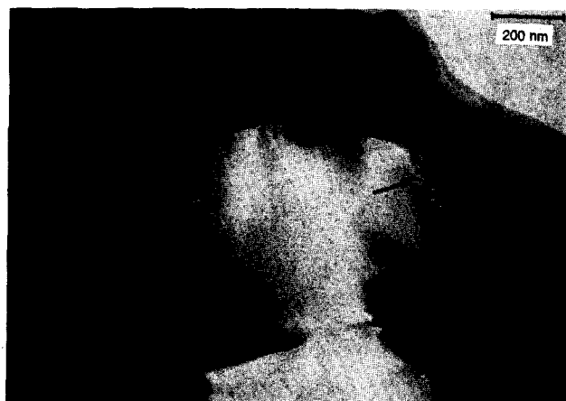
Fig. 3. Corroded SN1: 100 to 200 nm regions of foamed intergranular glass at a \text{Si}_3\text{N}_4 grain, and (smaller arrows) indications of general intergranular attack.
