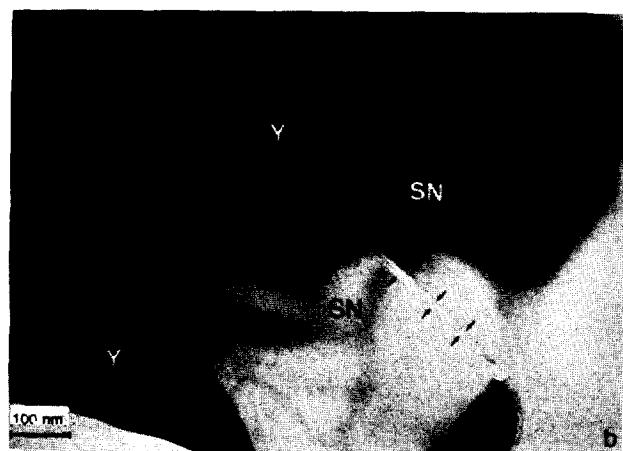
Fig. 4. (a) Nano-void formation at a silicon nitride-silicon nitride grain boundary; (b) complete grain face separation.
