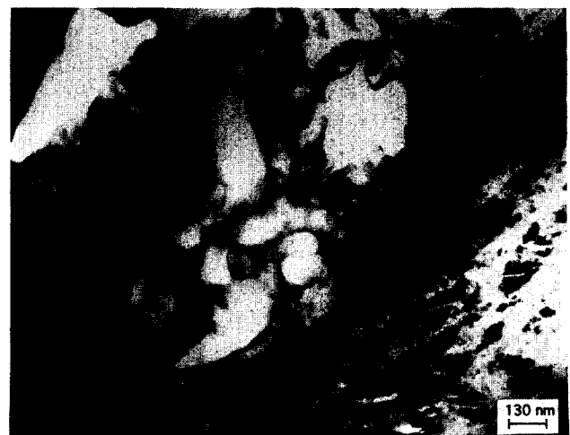
Fig. 13. TEM bright field micrograph of the fibre-matrix interface in a 20 vol.% fibre composite sintered at 1600°C for 1 h.
