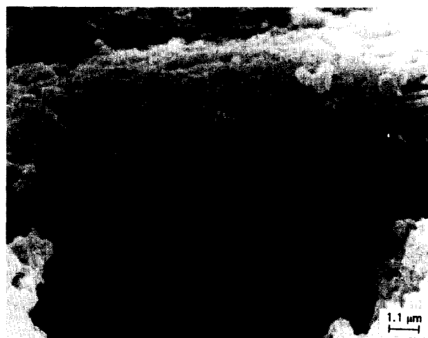
Fig. 5. SEM micrograph of the external surface of a reacted fibre in a 10 vol.% fibre composite sintered at 1600°C for 1 h.
