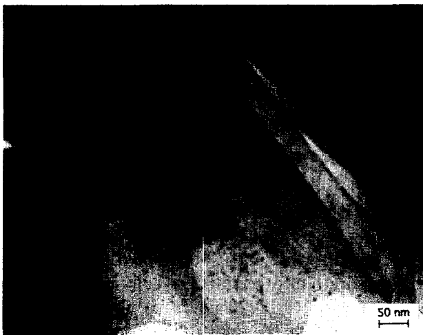
Fig. 17. TEM bright field micrograph of a 10 vol.% fibre composite sintered at 1600°C for 5 min.
