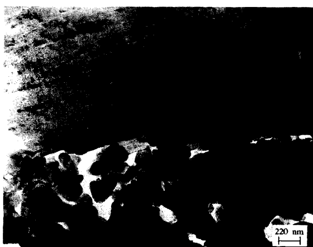
Fig. 9. TEM bright field micrograph of a fibre-matrix interface in a 10 vol.% composite sintered at 1500°C for 1 h.
