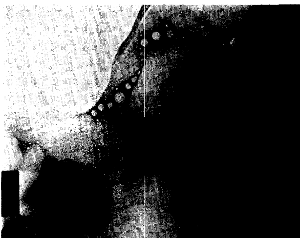
Fig. 18. TEM bright field micrograph of gas pores in the liquid phase of a 20 vol.% fibre composite sintered at 1600°C.
