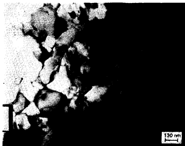
Fig. 8. TEM bright field micrograph of the matrix of a 20 vol.% fibre composite sintered at 1600°C for 1 h.
