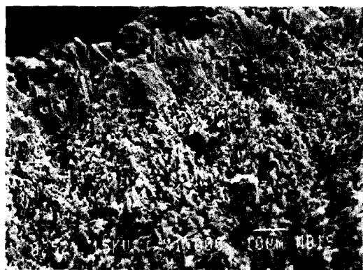
Fig. 14. Cross-section of the oxidized scale in the case of oxidation perpendicular to the pressing axis. Presence of a dense liquid layer.
