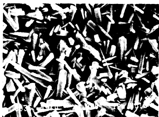
Fig. 15. Oxidized scale for oxidation parallel to the pressing axis: A9B2 crystals and open porosity.
