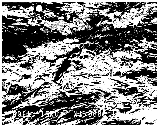
Fig. 3. Fracture faces of an undoped composite with an important porosity due to a bad BN platelets orientation.
