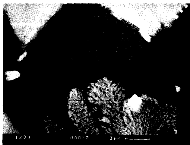
Fig. 6. Y–Al–Si-rich phase at 1200°C with part of a \gamma - \text{Y}_2\text{Si}_2\text{O}_7 loose network and Y–ZrO 2 particles (backscatter image — 5000×).
