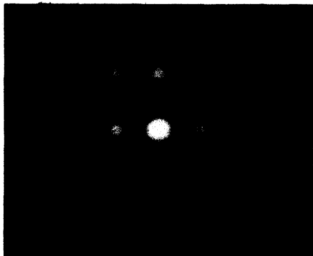
Fig. 15. ( h0l ) reciprocal lattice section of as-sprayed 2/1-mullite, displaying sharp and diffuse reflections as well as diffuse streaks in an a^*/c^* plot. The diffraction pattern was obtained from the mullite core grain shown in the inset of Fig. 4.
