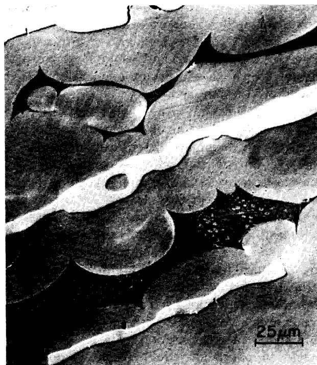
Fig. 4. Microstructure of specimen containing 71.8 wt% \text{Al}_2\text{O}_3 held at 1950°C for 7.7 h, cooled to 1750°C in 30 min, annealed at 1750°C for 29.4 days, and quenched to room temperature. Light grey precipitates are alumina completely surrounded by layer of mullite. Dark grey portions between mullite layers are glass containing precipitates of mullite formed on quenching. The microstructure formed during the heating schedule indicates a peritectic reaction.
