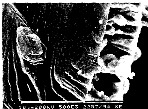
Fig. 6. High frequency sputtered ZrO 2 layer (4 h) on single crystal \alpha -Al 2 O 3 fibre, after reaction bonding at 1500°C.
