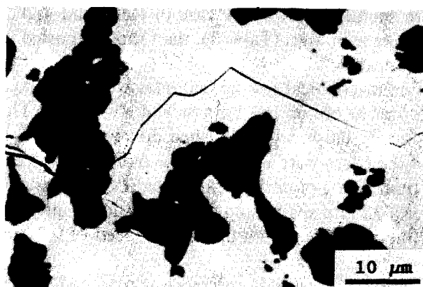
Fig. 4. Backscattered SEM micrograph of ER RS Si-SiC composites; polycrystalline silicon carbide (35 vol%). Crack moves mainly in silicon region and is deflected by SiC grains.
