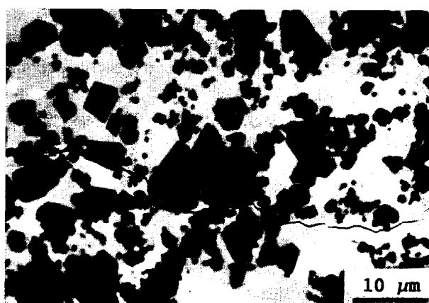
Fig. 5. Backscattered SEM micrographs of ER RS Si-SiC composites; polycrystalline silicon carbide (50 vol%). Also, at this SiC content, the crack moves mainly in the silicon region and is deflected by SiC grains.
