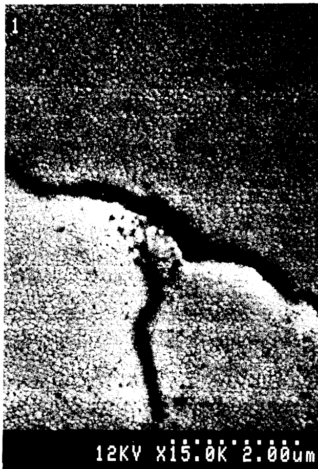
Fig. 7. Microstructure of the HC-W material sintered at 1050°C for 5 h showing a crack.
