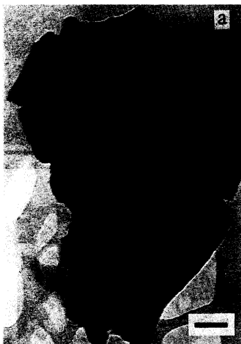
Fig. 11. TEM micrograph of sample B dried gels; bar = 50 nm.
