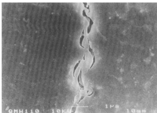
Fig. 10. Secondary cracking and the formation of crack wedges during cyclic loading.
