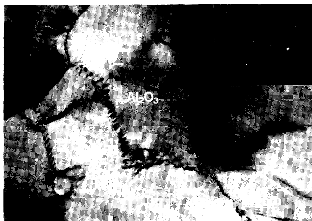
Fig. 12. TEM micrograph of \text{Al}_2\text{O}_3 feature showing low-angle \text{Al}_2\text{O}_3 – \text{Al}_2\text{O}_3 grain boundary and high-angle \text{Al}_2\text{O}_3 –Al grain boundary. Diffraction pattern shows \text{Al}_2\text{O}_3 [006].
