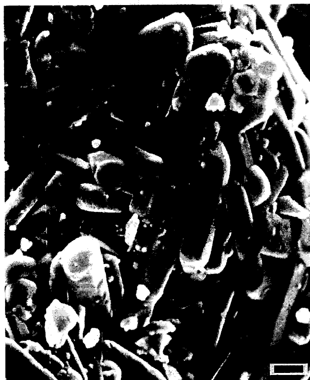
Fig. 5. SEM micrograph of sample B fired at 1400°C/96 h; bar = 1 μm.
