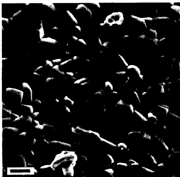
Fig. 4. SEM micrograph of sample A fired at 1400°C/96 h; bar = 1 μm.
