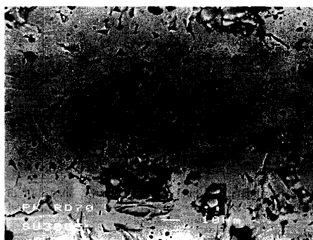
Fig. 2. Secondary electron SEM image of a tabular alumina grain well away from the corrosion front, showing its porous nature.
