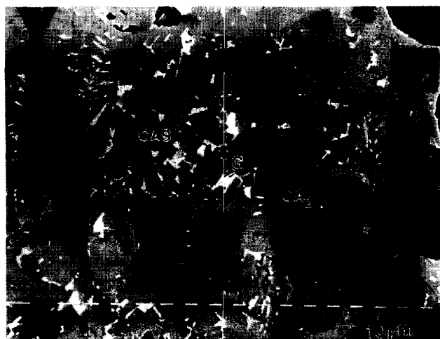
Fig. 7. Detail of the slag phases showing CA_2 needles, blocky spinel (S), calcium aluminosilicate (CAS) matrix and bright phase G whose triple junction morphology suggests it is the last phase remaining after crystallization and may well be glass.
