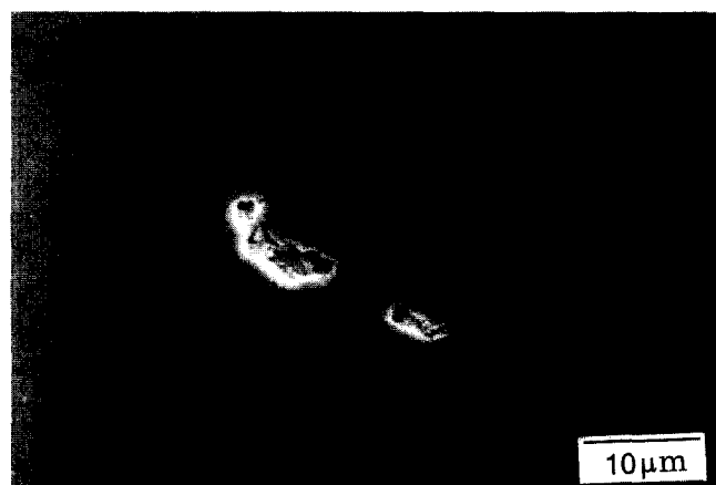
Fig. 8. Defect found in 98% dense hydrothermally crystallized (HC) material.
