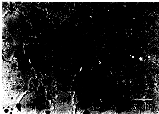
Fig. 9. Microstructure of HIPed (Mg,Y)-PSZ with 3 vol% \text{MgAl}_2\text{O}_4 spinel. Spinel particles appear within the pore-free bulk as black.
