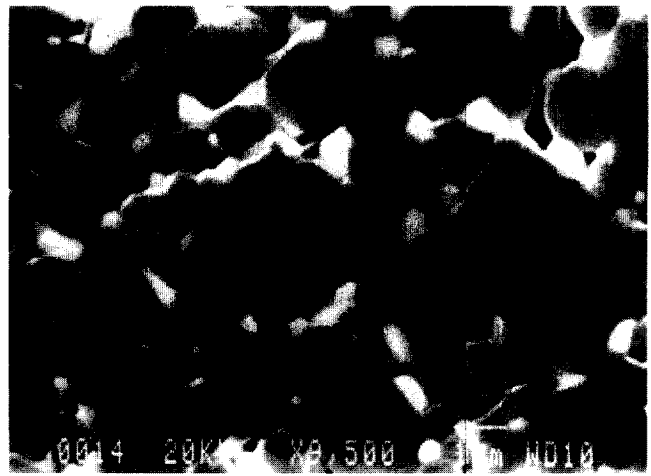
Fig. 7. Microstructure of Al-10Zl composite crept at 1200°C, showing the presence of numerous cavities.
