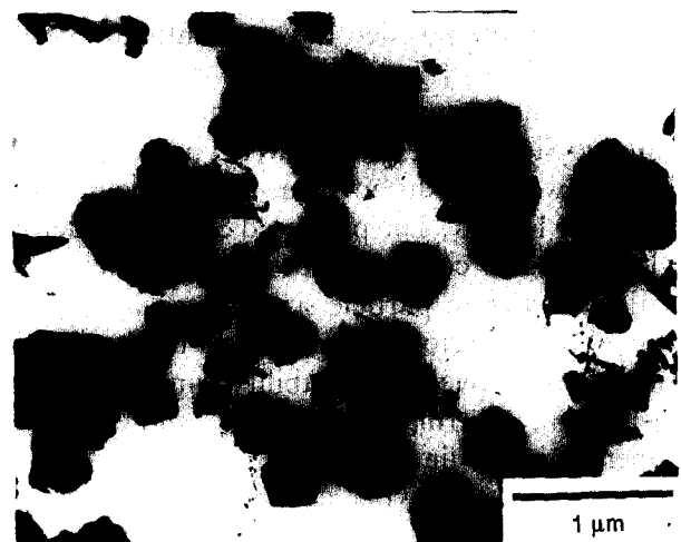
Fig. 7. TEM micrographs of produced powders from seeded precursors at 1500°C for 5 h in flowing nitrogen gas.
