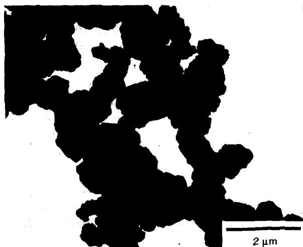
Fig. 8. TEM micrographs of produced powders from mixed precursors at 1500^\circ\text{C} for 5 h in flowing nitrogen gas.
