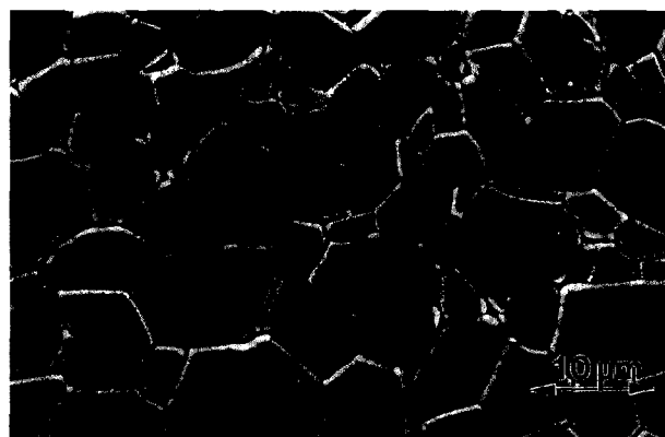
Fig. 3. Sample SEM micrograph of 8.5 \mu\text{m} grain size material following thermal etching showing equiaxed grain morphology.
