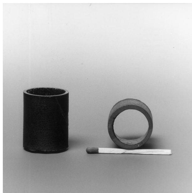
Fig. 2. Some examples of SiC/graphite laminated tubes consisting of 19 SiC layers (95 ± 12 \mu m) and 18 graphite layers (10 ± 3 \mu m). The outer diameter is 23 mm; the inner diameter is 19 mm and the length of the standing tube is 35 mm.
