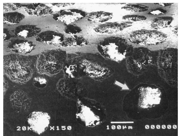
Fig. 10. Microstructure of a composite made with TCP granules presintered at 500°C but subsequently impregnated with Vaseline to make them unwettable.
