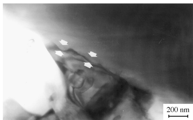
Fig. 4. TEM observation of the platelet–matrix interface probably showing the presence of graphite.
