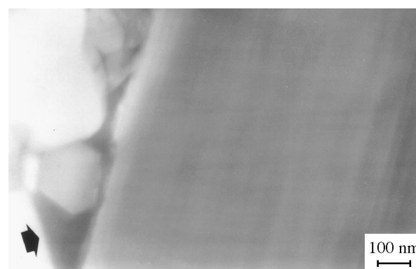
Fig. 3. TEM observation of the platelet–matrix interface showing glassy phase.
