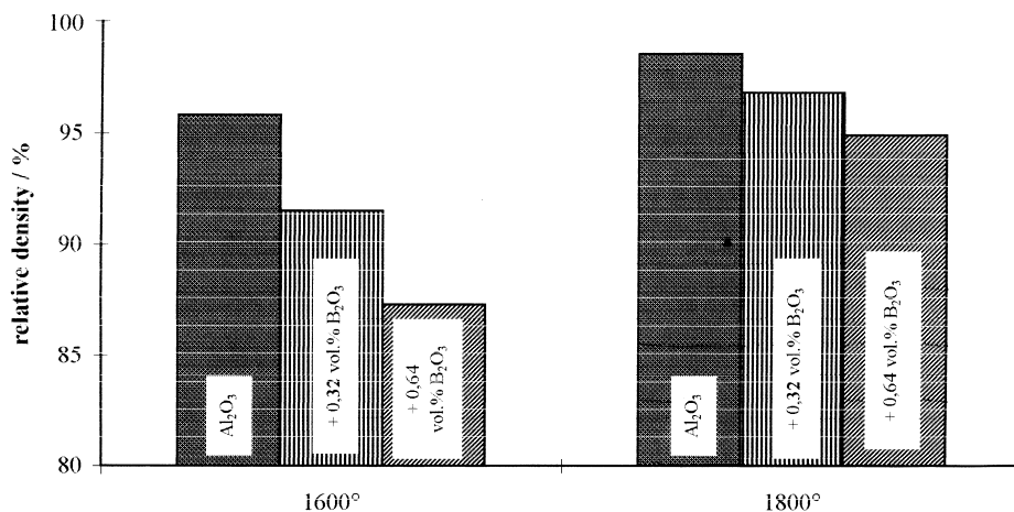
Fig. 8. The influence of B 2 O 3 on the density of Al 2 O 3 after firing at 1600 and 1800°C (heating rate: 10 K/min; no soaking time; atmosphere argon).
