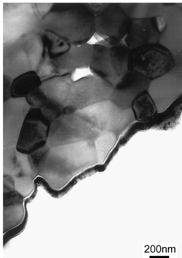
Fig. 5. TEM image of amorphous LaVO 4 PVD coating as-deposited on FP (Du Pont)-Al 2 O 3 fibre.
