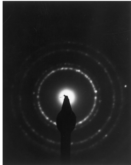
Fig. 11. SAED pattern obtained from the nanocrystalline phase in the annealed film.
