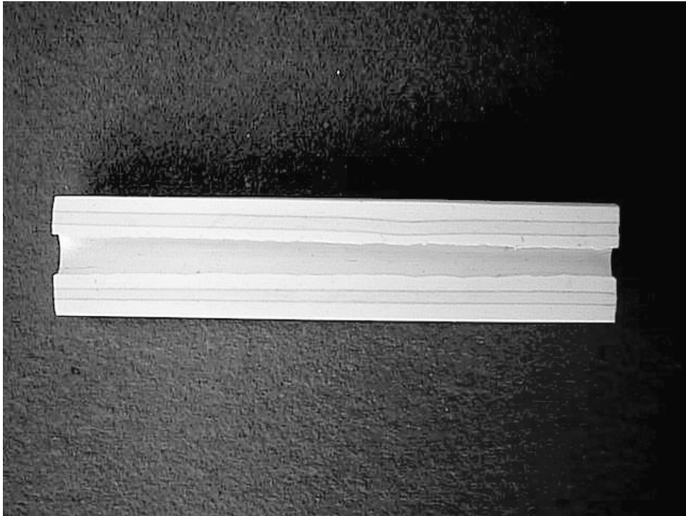
Fig. 5. \text{Al}_2\text{O}_3 /porous \text{Al}_2\text{O}_3 / \text{Al}_2\text{O}_3 trilayer tube fabricated in the co-extruder (outer diameter 6 mm).
