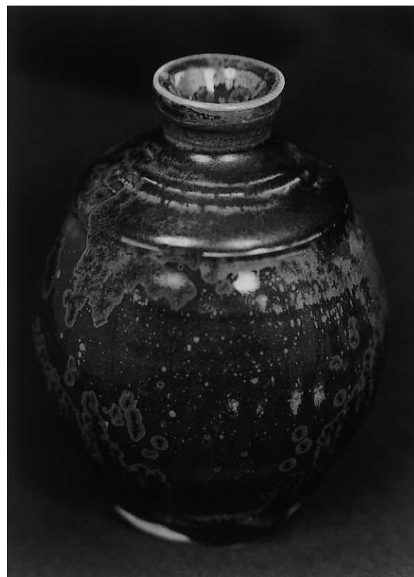
Fig. 10. A vase glazed with albite and 3% CoO containing glaze heat treated by HTC 2.
