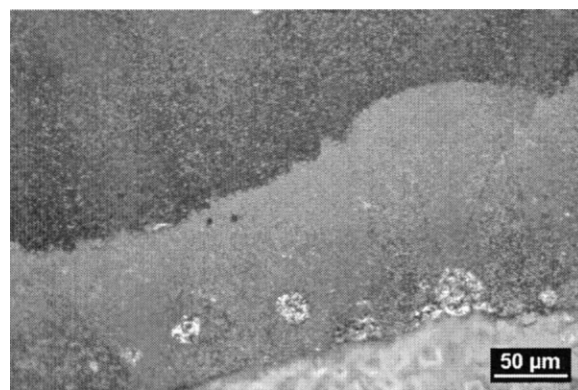
Fig. 2. Large grains near the \text{SiO}_2 tip, grown by anomalous grain growth.
