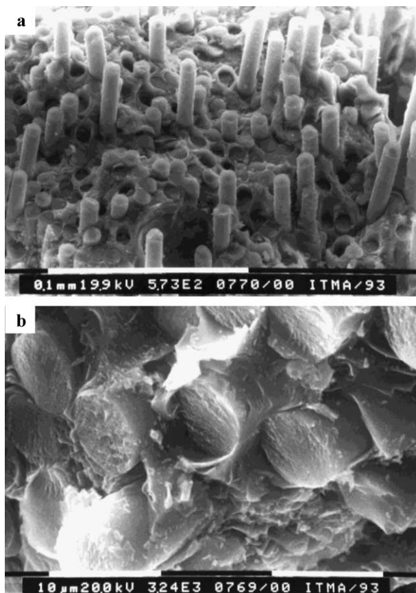
Fig. 11. SEM micrographs of fracture surfaces of composites: (a) C-DN0 and (b) C-DN5, illustrating fibre pull-out in the first sample and a more simultaneous failure of fibre and matrix for the latter.
