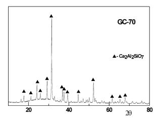
Fig. 2. XRD spectrum of the sintered glass-ceramic.
