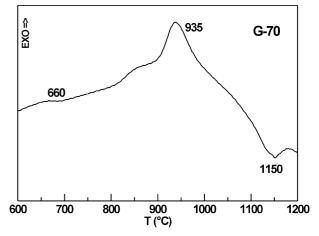
Fig. 1. DTA trace of the parent G-70 glass.
