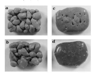
Fig. 3. Pictures of samples ( $3\times2$  cm) heat-treated at 2 °C/min and 1 h at 950 °C (a) and 1050 °C (b); samples heat-treated at 20 °C/min and 1 h at 950 °C (c) and 1050 °C (d).
