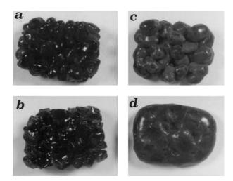
Fig. 5. Pictures of samples ( $3\times2$  cm) heated to 850 °C at 2 °C/min (a) and at 20 °C/min (b); picture of GC 2/20 (c) and GC 20/20 (d).
