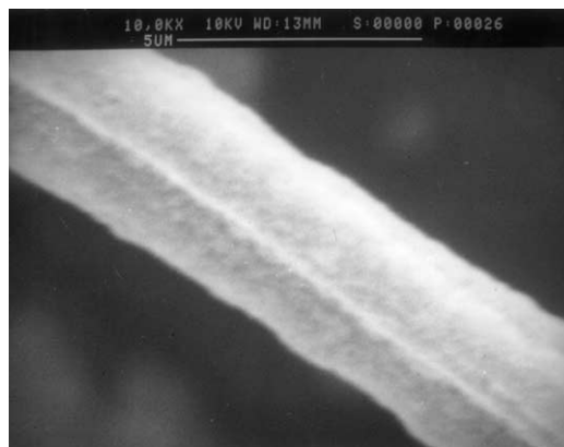
Fig. 7. SEM micrograph of a single strand of \text{GdFeO}_3 fibre.
