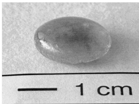
Fig. 2. Glass bead of the Lu-based glass after heat treatment at 1700 °C.
