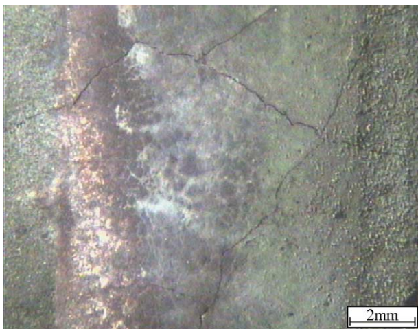
Fig. 5. An optical stereomicroscope image of the as-treated track of sample UP0850F25V3, showing the crack morphology.
