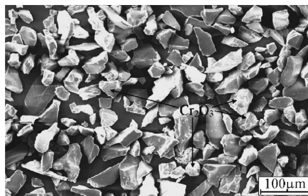
Fig. 1. A typical secondary electron scanning electron micrograph of the mechanically blended powder (20% \text{Cr}_2\text{O}_3 and 80% \text{Al}_2\text{O}_3 by weight).
