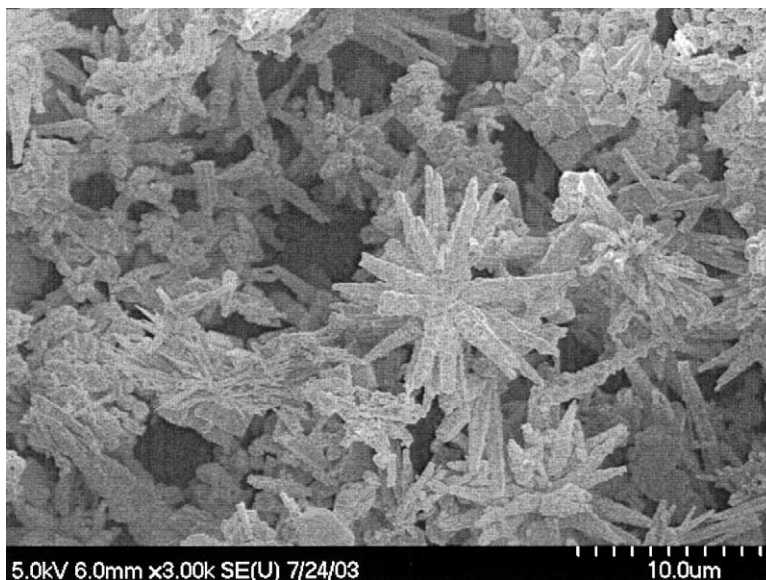
Fig. 5. SEM micrograph of the precipitate inside the cup during the hydrothermal reaction of Ba(OH) 2 and TiO 2 anatase with an OUT type setting. XRD shows that most of the precipitates are BaCO 3 .
