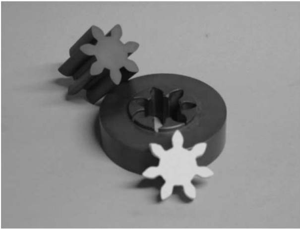
Fig. 8. Sinter formed gear (diameter 35 mm) and tooling (die and punch) made of SiC.
