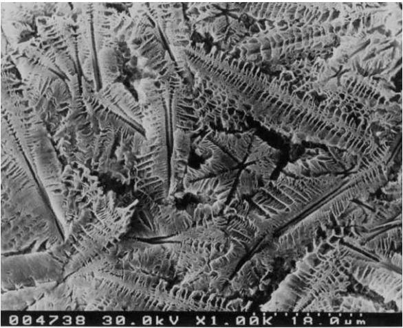
Fig. 12. FESEM micrograph of COMG glass isothermally treated at 900 °C for 264 h (bar = 18 μm).
