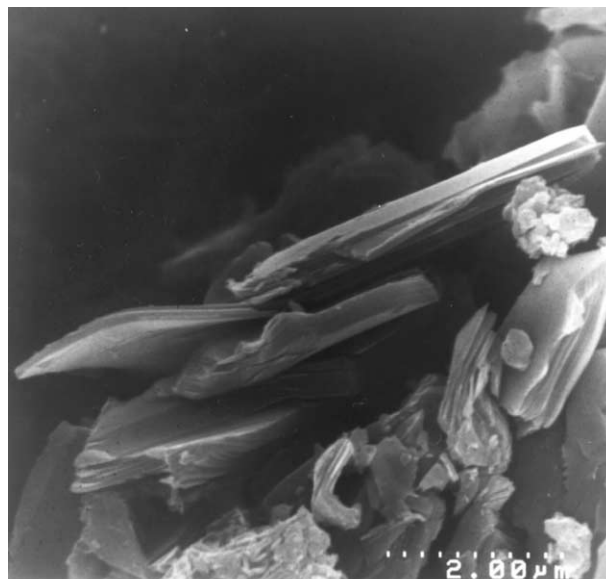
Fig. 5. The SEM micrograph showing the morphology of the powders of composition \text{Bi}_{1.6}\text{Pb}_{0.3}\text{Sb}_{0.1}\text{Sr}_2\text{Ca}_2\text{Cu}_3\text{O}_y (C1).
