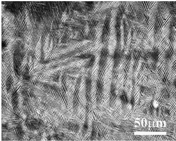
Fig. 3. OM image showing the domain configuration in a \langle 111 \rangle_{\text{cub}} -oriented PMN-PT single crystal sample.
