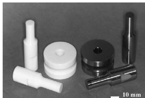
Fig. 1. 10 millimetre flat-faced F-tooling manufactured from zirconia and steel.
