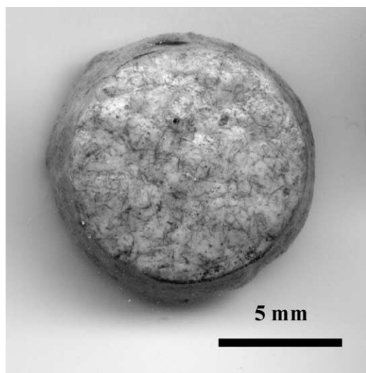
Fig. 2. Macrograph showing final shape of a foam borosilicate glass sample containing 10 vol.% Hastelloy X fibres after microwave processing.
