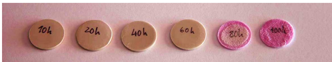
Fig. 2. Cylindrical samples fired at 1650 °C for different dwell times (10, 20, 40, 60, 80 and 100 h).
