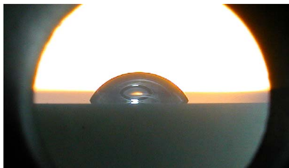
Fig. 2. Exemplary photo of a water drop carefully applied on the surface of a disk made of ZrO_2 ( \Theta = 65.1^\circ ).
