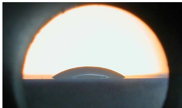
Fig. 3. Exemplary photo of a drop of anionomer 2a aqueous dispersion carefully applied on the surface of a disk made of Al_2O_3 ( \Theta = 36.1^\circ ).
