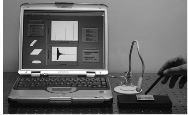
Fig. 8. Experimental set-up for the measurement of the resonance frequencies.
