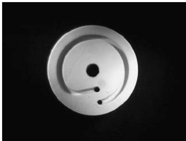
Fig. 6. Black and white photograph of a Möbius resonator synthesized from Zr- and Ni-doped \text{Ba}(\text{Zn}_{1/3}\text{Ta}_{2/3})\text{O}_3 using ceramic injection moulding. The sample itself has a light yellow color.
