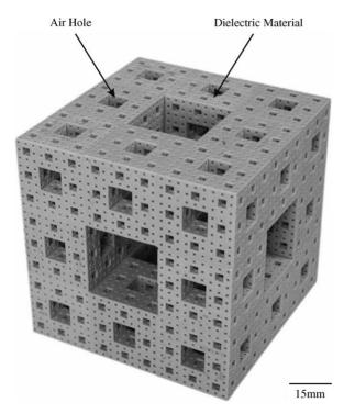
Fig. 3. A photonic fractal with the Menger-sponge structure composed of epoxy incorporating titania–silica dielectric particles.
