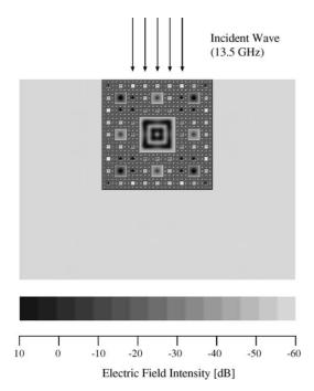
Fig. 5. An intensity profile of the electric field at the localized frequency inside and outside of the Menger-sponge.
