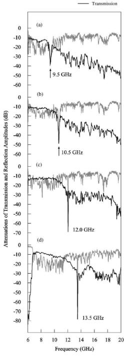
Fig. 4. Transmission and reflection spectra of the photonic fractals with the Menger-sponge structure: (a) stage 1; (b) stage 2; (c) stage 4; (d) stage 4.
