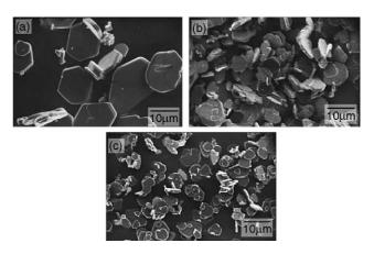
Fig. 3. SEM micrographs of powders obtained after heat treatment at  $1300\,^{\circ}$ C using (a) NaCl; (b) NaCl–KCl; (c) KCl.
