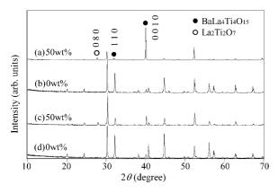
Fig. 4. XRD patterns of the (a, b) natural surface (c, d) polished surface of BLT prepared with plate-like crystal sintered at 1600 °C for 2 h.
