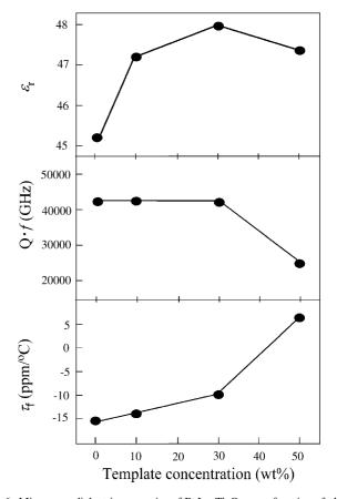
Fig. 6. Microwave dielectric properties of  $BaLa_4Ti_4O_{15}$  as a function of plate-like crystals in the starting mixture.
