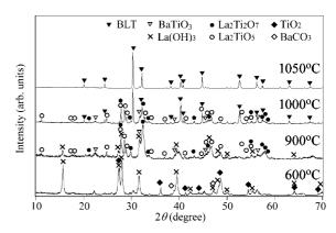
Fig. 2. XRD patterns of powders subjected to heat treatment at various temperatures for 2 h using NaCl.
