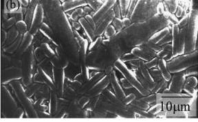
Fig. 5. SEM micrographs of the surface of the specimen sintered at  $1600\,^{\circ}\text{C}$  for  $2\,\text{h}$  (a) without and (b) with plate-like crystals. The pressing direction in normal to the plane of SEM picture.
