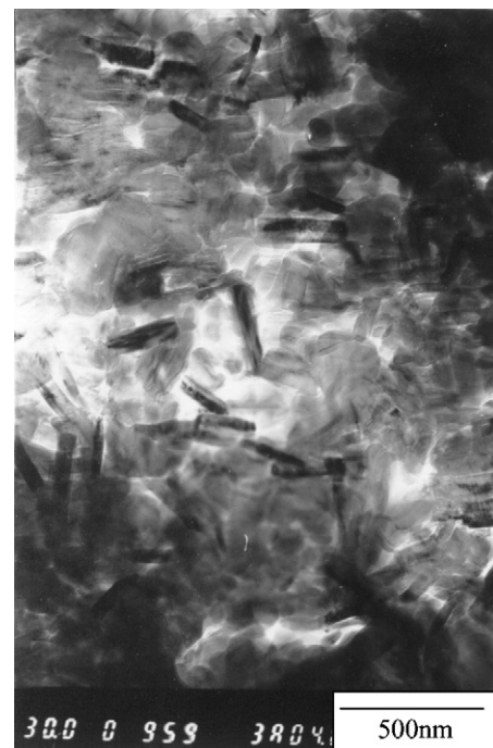
Fig. 12. Groups of nano-sized grains of BN agglomerates.
