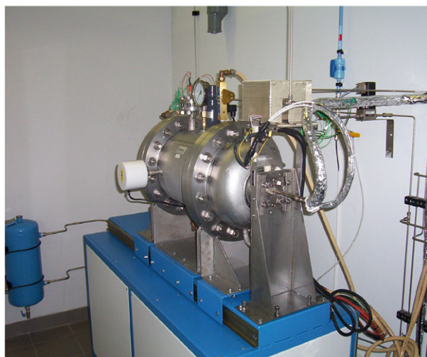
Fig. 3. Schematic of the high temperature–high pressure corrosion test equipment (a) and view of the furnace (b).
